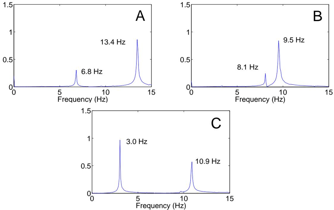
Figure 6: Frequency-domain of mixed low-energy signals at [A] 6.8 Hz and 13.4 Hz, [B] 8.1 Hz and 9.5 Hz, and [C] 3.0 Hz and 10.9 Hz
