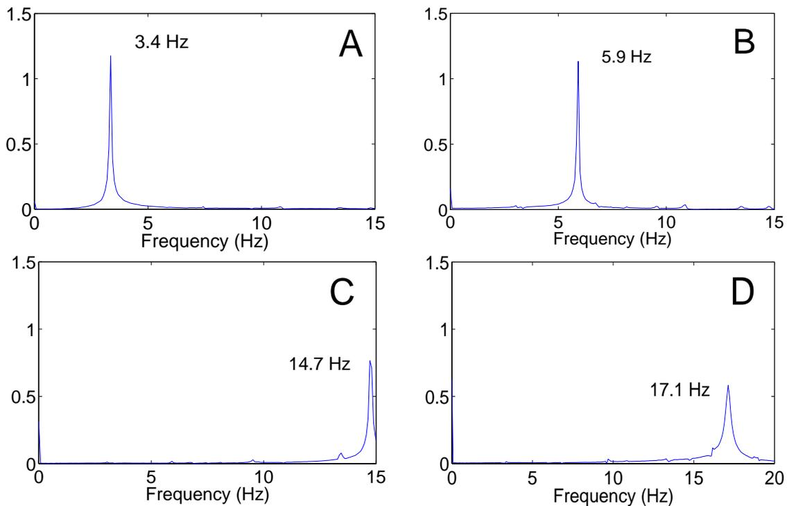
Figure 5: Frequency-domain of clean separated signals of [A] 3.4 Hz, [B] 5.9 Hz, [C] 14.7 Hz, and [D] 17.1 Hz
