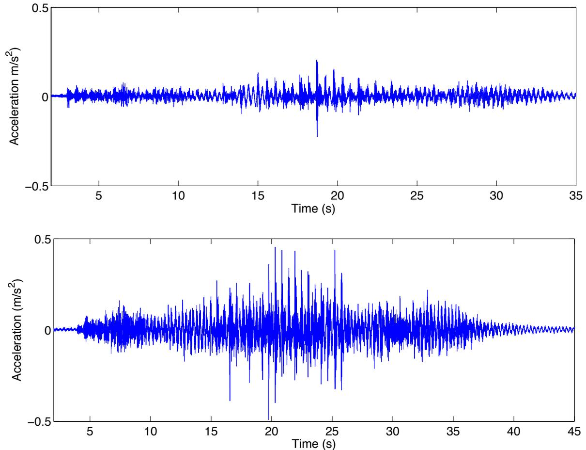
Figure 8: Response at location B (centre) of the bridge for [A] a single person walking and [B] group of 5 people walking
