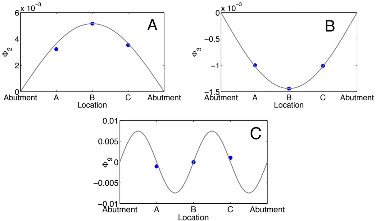
Figure 7: Mode shapes for [A] 3.0 Hz vertical, [B] 5.9 Hz vertical-torsional, and [C] 14.7 Hz torsional
