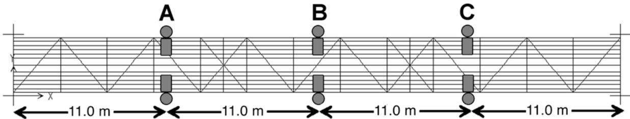
Figure 2: Plan view of PCB wired accelerometer locations installed on bridge girders
