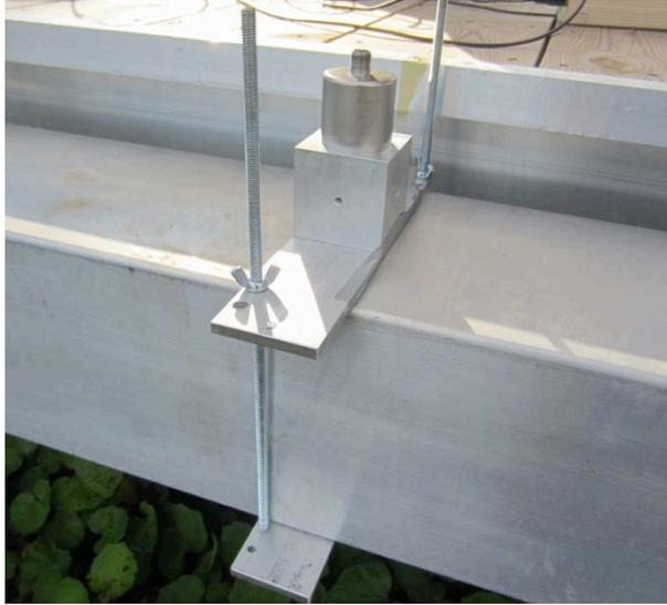
Figure 3: Installation of vertical accelerometer on the bottom square girder of the bridge using a sandwich-style clamp
