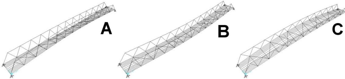
Figure 4: Finite element first mode shape for [A] 3.1 Hz lateral-torsional, [B] 3.4 Hz vertical, and [C] 5.6 Hz vertical-torsional
